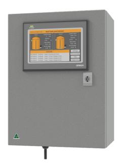
MATelec Australia's advanced dual tank level indicator has been designed to provide the ultimate in accuracy, flexibility and additional control for maintaining levels of up to two tanks. With a comprehensive touch screen interface, on board data logging, programming for vessel shape, expandability via RS485 and multiple relay outputs making this the pinnacle of tank level indication.
