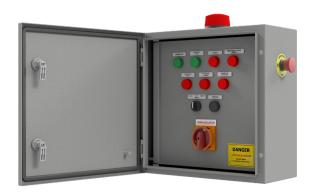
The Macerator Controller has been specifically designed for the processing of waste in the sewage industry. The controller uses current sensing to detect an overload of a grinder due to an obstruction. To attempt a clearance of the blockage, the controller will engage the grinder to run in reverse for a period before returning to the forward direction.
