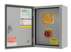
The unique Deluxe Rain/Mains Valve & Pump Controller is the market lead in rainwater use prioritisation and maximisation. Designed to provide a continuous supply of water by monitoring the level in a tank and providing power and control to a pressure pump. When tank water is depleted or in the event of a mains power failure, the system will close the main rainwater supply valve and deactivate the pump to allow mains water to flow into the system.
