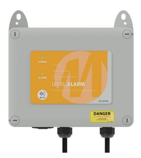
The Under Sink/Sullage Alarm and Dishwasher Interlock has been specifically designed to monitor the level in an under sink sullage tank. If it detects the tank level full, possibly due to pump failure, the control will shut the mains supply to the Dishwasher in the system, ensuring no further water can enter the sullage tank.
