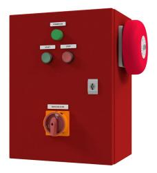
The Residential Sprinkler Pump Controller gives control and status indication for one or two residential sprinkler pumps. Compliant with the current Australian Standards (AS 2941-2013: Section 7), the Residential Sprinkler Controller features push buttons for manual start and stop, pressure switch inputs for automatic control and an audible alarm via an electronic bell that sounds while pumps are running.
