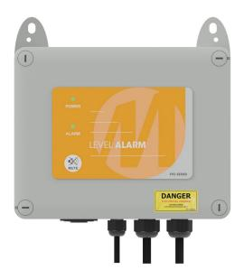
The Standard Under Sink/Sullage Alarm with Valve Shutoff monitors the level in an under sink sullage tank and in the event that the tank level goes full, possibly due to pump failure, the control will shut the mains water supply valve and give an alarm signal.
