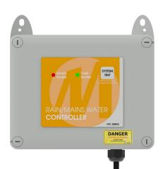
The Standard Plus Rain/Mains Valve Controller builds on the capabilities of the standard version. The Standard Plus comes with an additional special purpose outlet that can be employed to power an automatic pump and create a fully automated system. An additional input can be used for a pressure switch and allow for the system to detect a fall in pressure within the system and close the valve.
