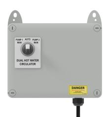
Designed to provide constant circulation of hot water through a supply system, the Standard Hot Water Circulation Panel alternates the pumps on a 4-hour cycle. The onboard time clock can be reconfigured to change the duty alternation period.
