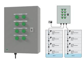
Designed to provide accurate indication up to four levels within a vessel. The Four Level Indication Panels use input control switches to indicate if the level of the vessel is above or below a set point and illuminate indicator lights for each set-point. These units provide optimum reliability and repeatability and are available in both single and dual tank variations.
