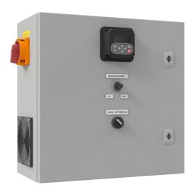
Available in three phase only, the Standard VSD Motor Controller can be configured for manual or automatic operation of a large VSD motors or pumps. Featuring additional functionality including overload protection, under/over voltage protection, phase failure, short circuit protection, a Potentiometer for adjustable speed control, as well as the standard inputs for a working and stop set point, these highly versatile controllers are ideal for many applications.
