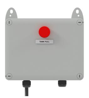
The Tank Fill Pump Controller has been specifically designed to operate in conjunction with an automatic pump. Featuring a float switch input to deactivate supply to the pump once the tank is full, these simple, yet effective controllers ensure that reservoirs, tanks or other storage vessels can be kept at their optimum level.
